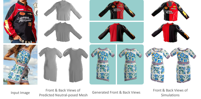
Fig. 7. Limitations. OmniFabric may synthesize mismatched textures from inaccurately generated multi-views (1st row), or generate garments with incorrect geometry even though appearance is well-transferred (2nd row).
